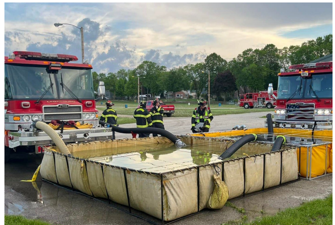
Training in May for Rural Water Supply, using two engines and 2 portable tanks.
